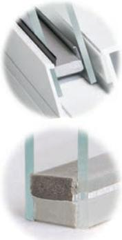
**The Intercept Warm-Edge Spacer** features a unique, one-piece metal alloy, U-channel design that reduces heat loss through the window. It's stronger and better at retaining insulating gas than many conventional spacers, and is nearly 25% more effective than a traditional metal spacer at the edge of the glass unit.
