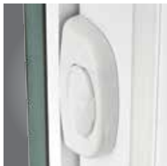
The positive action lock (PAL) ensures easy operation. A simple movement of the locking tab allows the sash to move freely; the PAL system locks automatically when the window is closed.
