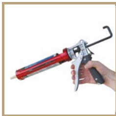
Caulking gun and caulking
