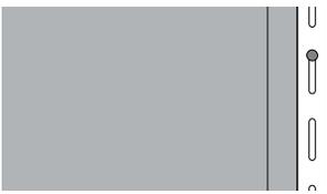
Fasten at the top uppermost unobstructed nail slot on the panel towards the top of the wall. DO NOT fasten through nailing flanges or any other accessories.
