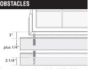
Place tape measure into the backside of the receiving channel, measure to the top of the plank face of previously installed plank (past nail hem). Transfer measurement plus 1/4" to the siding plank, pull tape from bottom of plank, mark and cut
