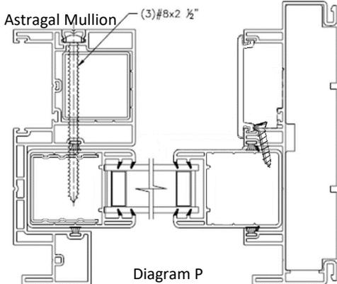
For regular fixed panel, follow the same procedure as with 2 panel doors. The fixed panel adapter on this side is 1/2" shorter than on the dummy panel side.
