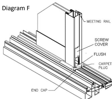
Tap the screw covers at the top and bottom of the free end of the fixed panel up and down against the head and sill. **The plain cut cover at the sill should finish on top of the Fixed Panel End Cap as shown on Diagram F. If it slides downwards beyond the end cap, this indicates that the fixed panel is not fully engaged into the jamb. Re-install the fixed panel if necessary.**
