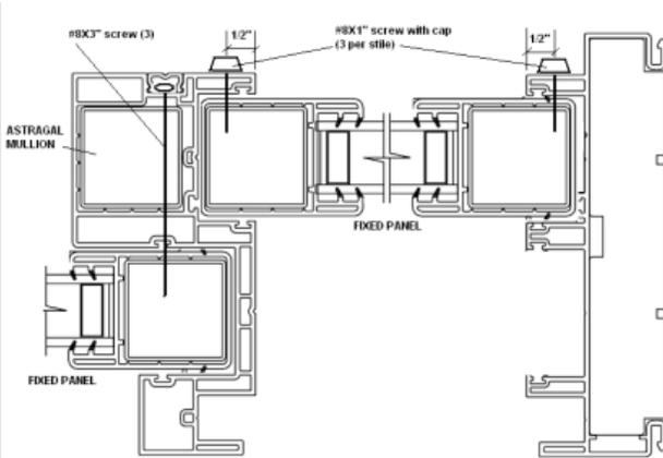
Locate the jamb side fixed panel without hardware on the inner sliding track, adjust the wheels to align the panel vertically to the jamb (see Diagram H), and slide the panel fully into the jamb pocket. Secure the panel to the jamb through the holes with 3 - #8 X 1" screws and screw caps provided as shown on Diagram S.
