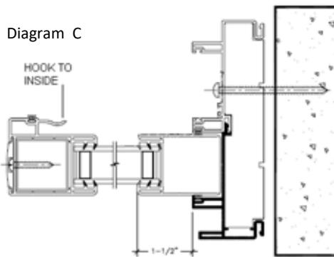
The fixed panel is supplied with screw covers at the top and bottom of the meeting rail. The plain cut cover is to be located at the bottom of the panel and the notched cover is to be located at the top. Remove and reverse to suit your door handing if necessary. Slide the screw covers away from the top and bottom of the meeting rail before installing the panel into the frame.
