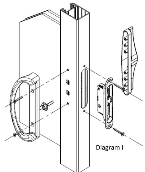
To locate the latch keeper on the jamb, open the operating panel, nest the keeper into the opening on the lock mechanism, and engage the thumb turn to hold the keeper within the lock mechanism. Apply a piece of 2-sided tape to the back of the keeper and firmly close the panel into the jamb. Disengage the thumb turn and slide away the operating panel. The latch keeper should be held in the jamb by the 2-sided tape. Mark the keeper location with a pencil and remove the tape.
