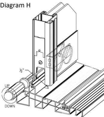
Using a hand-held screw driver, adjust the rollers up or down so that the exterior bottom of the panel is riding 1/2" above the sill. See Diagram H. Turn the screw clockwise to raise the panel or counter clockwise to lower the panel as shown on Diagram H. NOTE: We recommend lifting the panel slightly when adjusting the wheels for ease of turning and to prevent thread stripping the adjustment mechanism.
