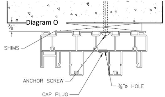
Use solid shims and ensure that the head is not bowed or twisted by the installation screws. Check for straightness and squareness before proceeding further. After installing the screws, apply urethane sealant around the hole and install the cap plug. Wipe clean any excess sealant.
