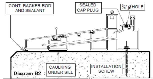
The use of cap plugs is recommended for aesthetic reasons to fill the  $\frac{3}{8}$ " diameter screw head clearance holes and to conceal the installation screws. Cap plugs and exposed screw heads must be fully sealed and water tight. All screws must engage the surrounding structure a minimum of 1".
