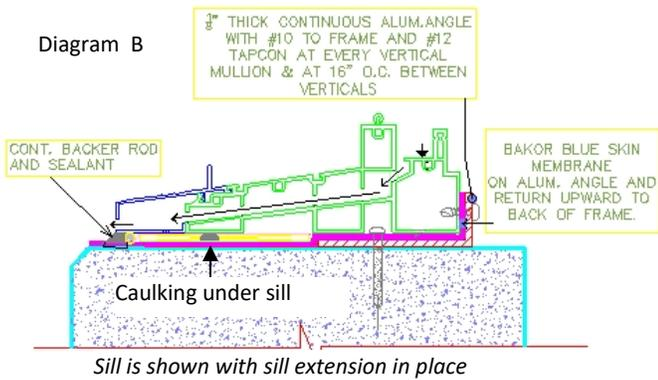
subfloor. Diagram B shows the recommended configuration to install the sill.
