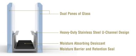
**Moisture Vapor Shield** BarrierXP ThermD Intercept Stainless Steel Spacer with a moisture-absorbing desiccant is stronger by design and better at retaining insulating gas compared to traditional box metal spacers; the moisture barrier also helps prevent the passage of water or water vapor that could fog the unit.
