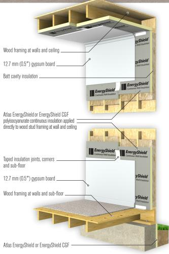
WOOD OR METAL FRAMING, BATT INSULATION IN THE STUD CAVITY, RIGID FOAM INSULATION FINISHED WITH 12.7 mm (0.5") GYPSUM THERMAL BARRIER
