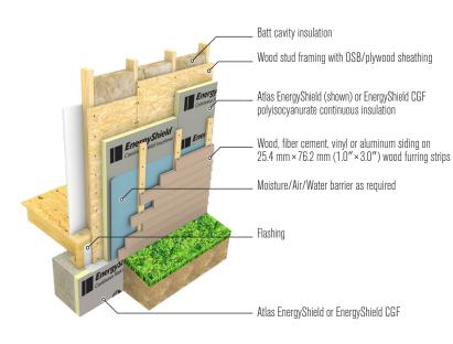
WOOD FRAMING, WOOD SHEATHING, CONTINUOUS INSULATION, AIR/MOISTURE BARRIER WITH CLADDING OVER FURRING STRIPS
