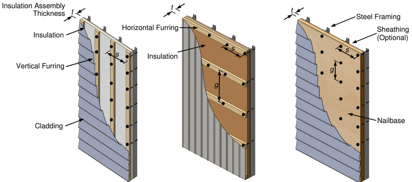
Figure 3: TRUFAST SIP LD into Cold-Formed Steel Studs
