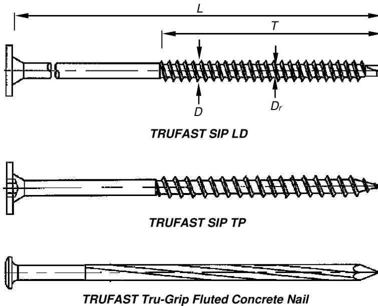
Figure 1: Fastener Geometry
