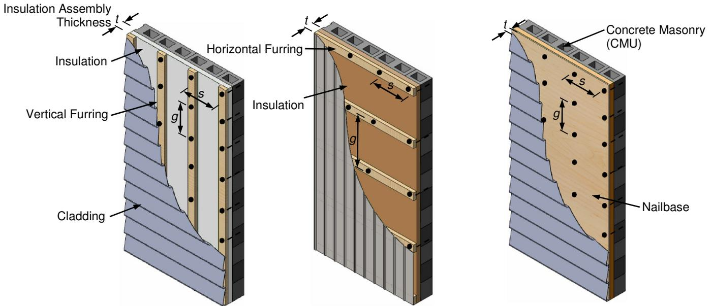
Figure 5: SIP LD into Concrete Masonry (CMU)
