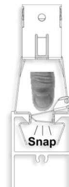
Spline Connectors are used to connect Dauntless Beams together to achieve a seamless look for linear runs greater than 24'. A 1/8" Hex Key is used (by others) to tighten the Set Screws once in the desired position. Spline Connector and Set Screws are purchased separately.
