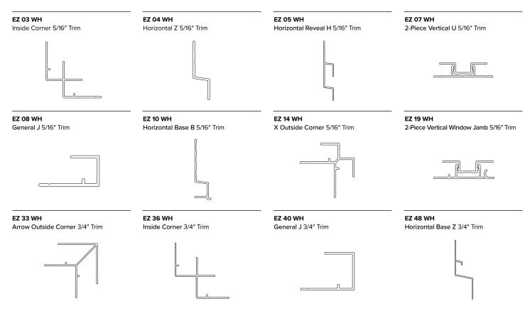
We offer a limited profile selection in the 5/16" and 3/4" series. Other profiles can be ordered with extended lead times.
