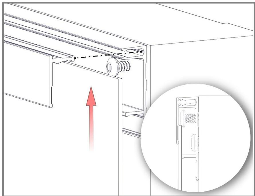
Step 10 - Once planks are installed, finish off the perimeter trims with caps from two-piece sets.
