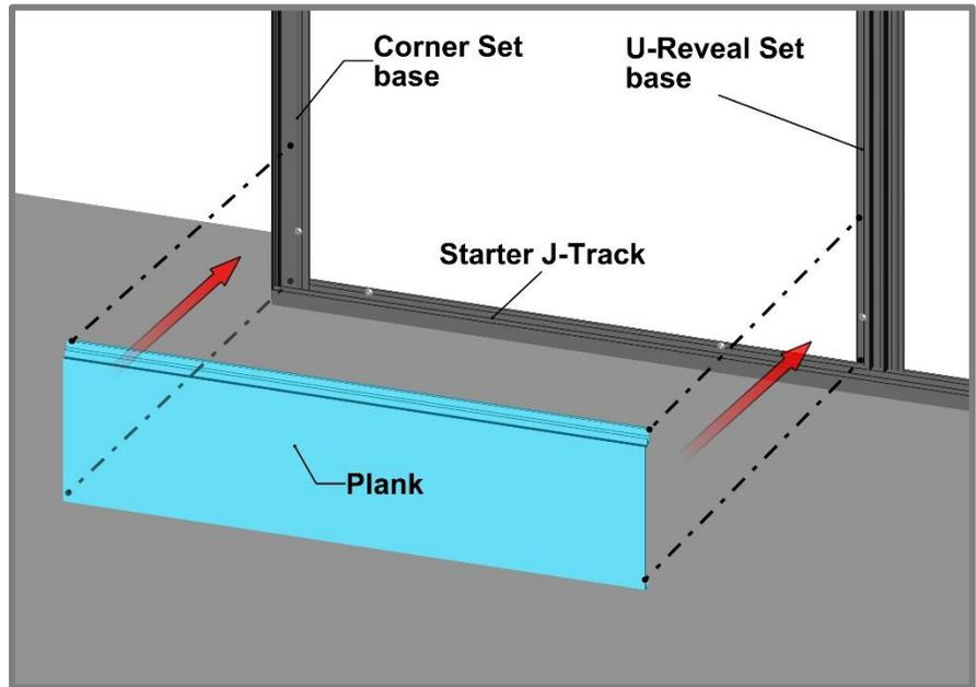
Ensure there is sufficient room for expansion and contraction of each Plank, also confirming component caps will cover.
