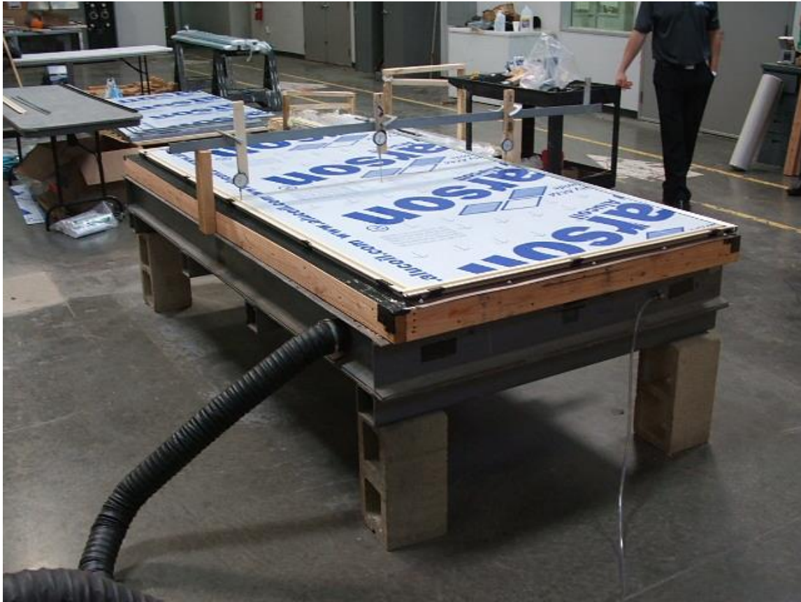
Photograph No.1 Negative Uniform Load Test Set-up
