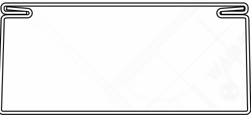
STANDARD EXPOSED LOCK SEAM ADHESIVE FILLED
