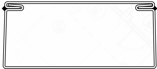
LOCK SEAM CONTINUOUSLY WELDED ENTIRE HEIGHT OF DOOR GROUND SMOOTH & BODY FILLED SEAMLESS EDGE
