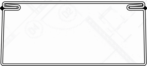
EXPOSED LOCK SEAM TACK WELDED
